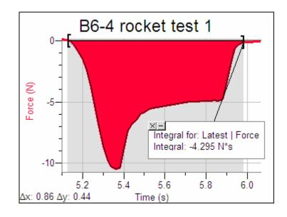
Mass of new motor: 17.1 gMass of used motor: 9.7 g
