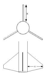
The coefficient of drag,  $C_d$ , is a dimensionless quantity (not unlike the familiar  $\mu$  from our friction problems) and is usually found through testing in a wind tunnel. It can be estimated mathematically but it is a complicated calculation. For our purposes, and without any better information, we will estimate it to be 0.75.
